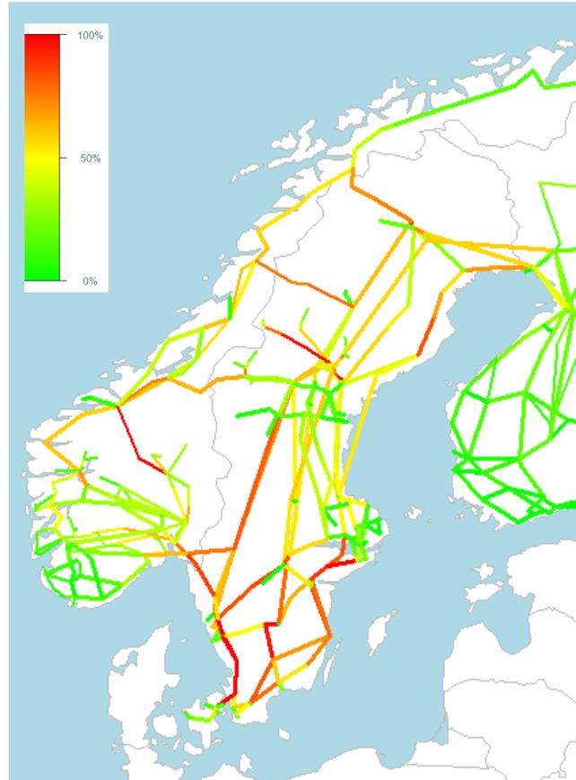
Line utilization in 2030 with increased capacity on all lines
